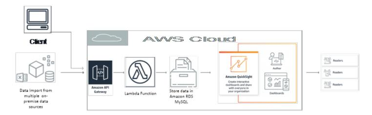
Currently, Amazon RDS is used as the dataset source, which suffices for reporting and analytical dashboard needs. A redesign using Amazon Redshift and AWS Glue is under trial for a complete enterprise analytical solution
